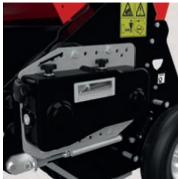
Easy to adjust seed rate gearbox.
