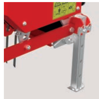
Storage legs for easy mounting and dismounting.
