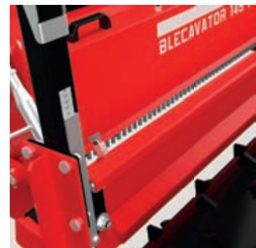
Levelling bar to create a smooth and level finish.
