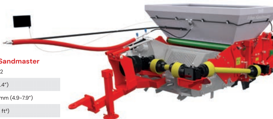
Adjustable coulters ensuring the correct amount of sand is delivered.
