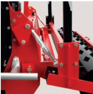
Moveable rear packer roller.
