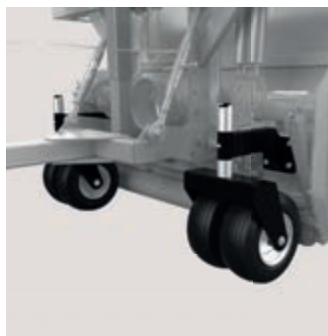
Optional caster wheels for hard surfaces.
