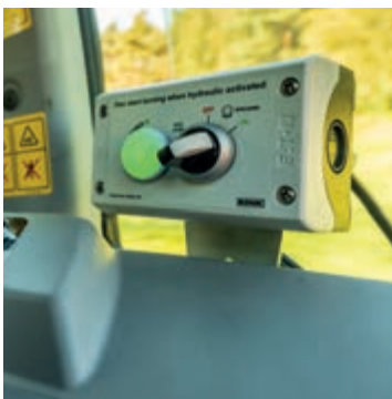
Analogue hydraulic flow control system.
