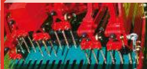
The turf hold down fingers ensure that, when verti-draining or coring, there is no danger of damage to the turf even with a shallow root system.
