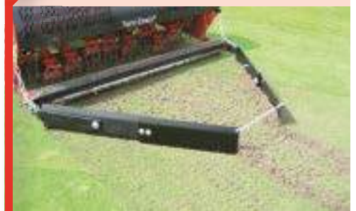
The Windrow kit aligns the cores for easy collection.
