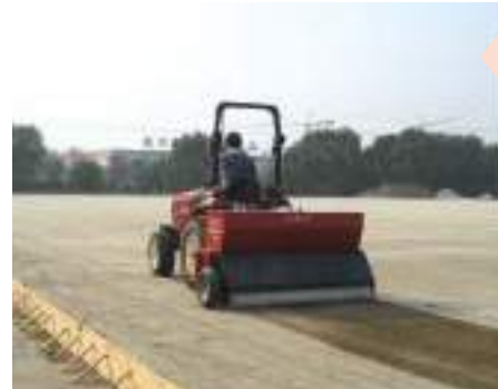
Sept 11, 2007 – The Olympic Grass, for the Beijing Olympics in august 2008, first being planted with the Speed-Seed, producing 1840 holes/m 2 for the seed to drop in.
