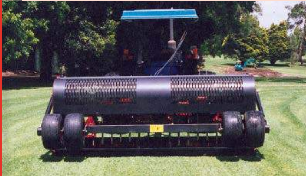
A retro-fit boggy wheel system is available for easy transport. This also means that a tractor with less lift capacity is required.
