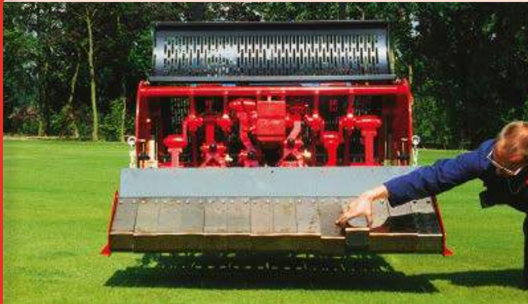
The Core Collector uses a flexible rubber flap to gather most of the cores. Behind there is a row of ground following aluminium fingers to ensure that all material is collected without the risk of damage to the turf.
