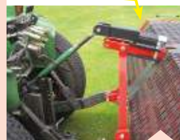
An optional anti-vibration system, containing a strong spring, can be added for stony conditions.
