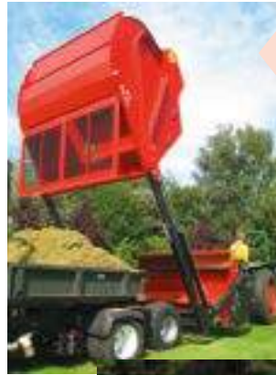
The tipping height of the hopper is 2.17m.
