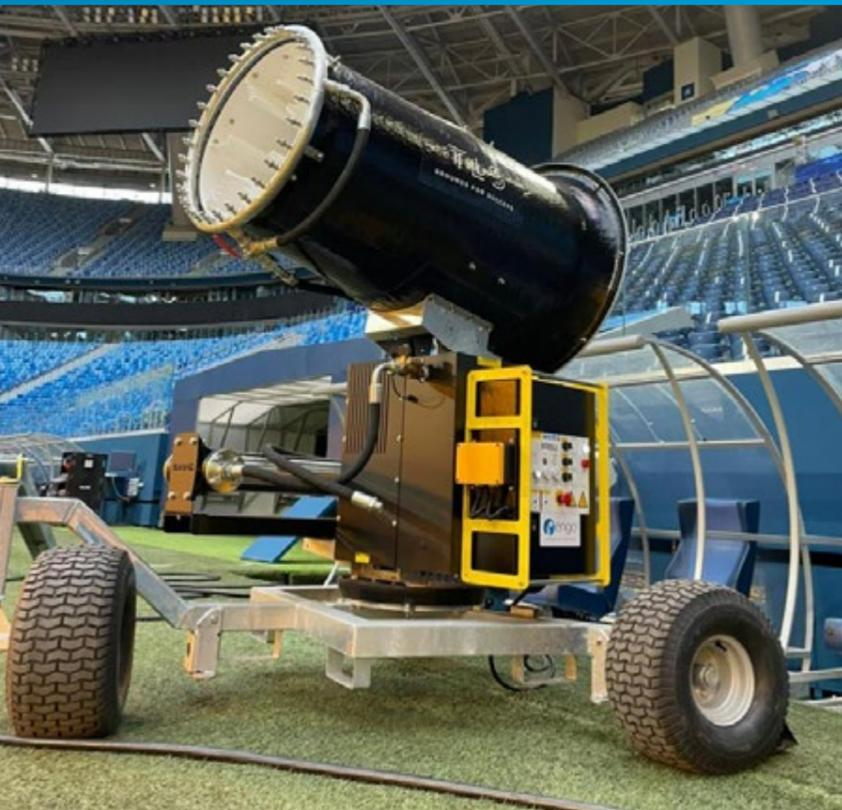
The TLS Turf Fan 510 series cools the air by means of mist in combination with a Fan. The grass cooling system consists of a fan and a micro mist system. The system can be used to ventilate only or to be combined with the misting system to cool the air for an improved environmental temperature to avoid stress to the grass.
