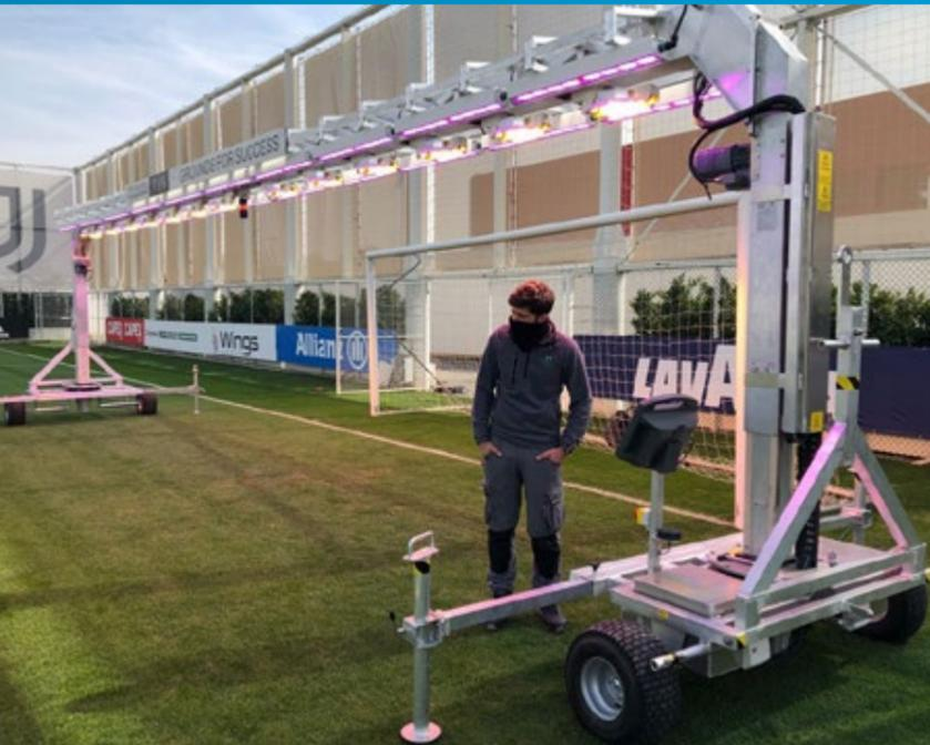
The TLS TurfLed 120 Hybrid comes with 20x 336 W HORTILED LED and 13x 1000W Hortilux HPS grow lights and covers an area of 120 m<sup>2</sup> at 420 μmol. It is height adjustable, can be set between 2.15 meters and 3.5 meters.
